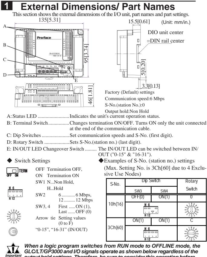
output hold settings. Therefore, be sure to consider this operation before resetting the unit or switching to OFFLINE mode.
